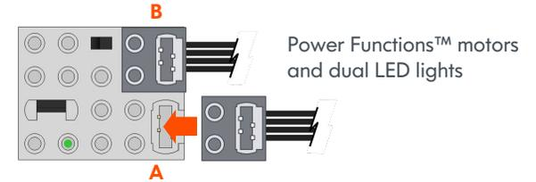
Connect any LEGO® Power Functions motor or LED accessory to the Pfx Brick Power Functions compatible outputs A or B located on top of the Pfx Brick.
