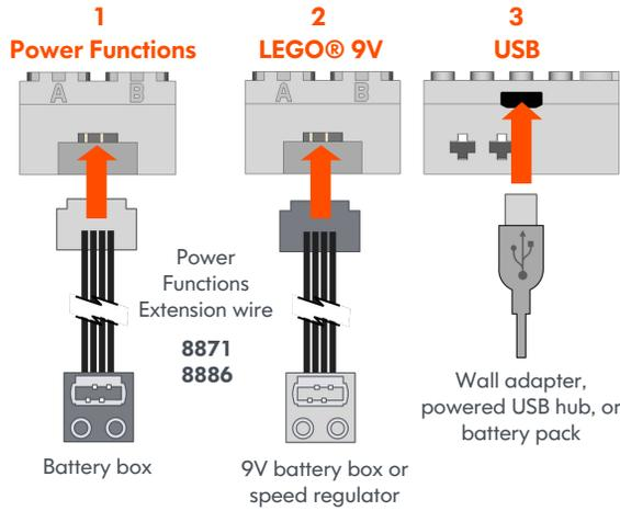
Battery box and USB power connections can be used simultaneously. The Pfx Brick will automatically use the best available power source.
