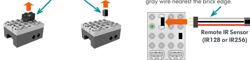
**!** Use caution when inserting/removing the IR sensor. The IR sensor pins are delicate and can be bent or damaged if mishandled.
