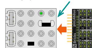
**!** If using the pinLABsolo, pinLABduo, or pinLABquad with Fx LEDs or OEM LEDs ensure the correct polarity of connection by matching the + label.
