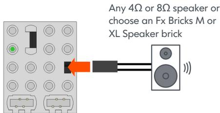
Connect speakers to the 2-pin female socket on the top of the Pfx Brick. Speakers can be connected in any orientation:
