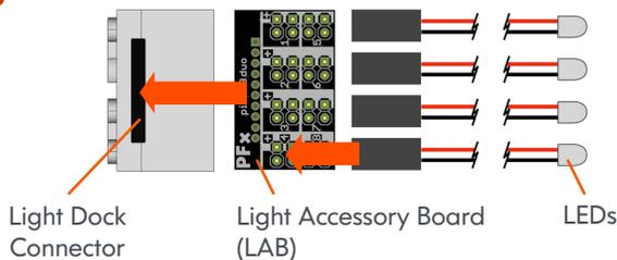
The Light Accessory Board (LAB) allows you to connect LEDs from a variety of manufacturers.
