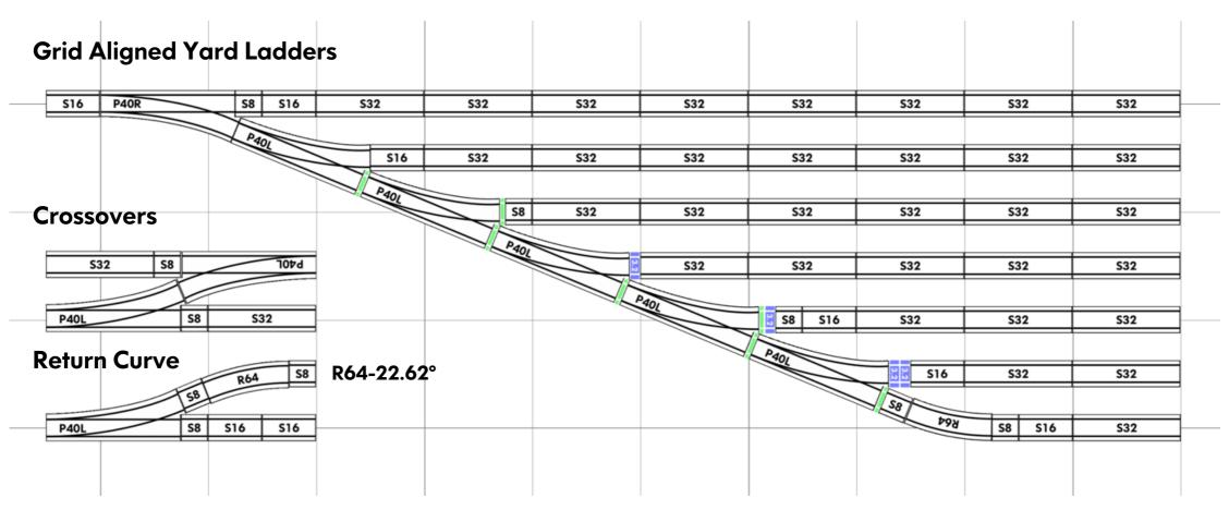
R64-22.62° ensures perfectly aligned return curves for parallel sidings with Right/Left/Y switches and for yard ladder terminations
