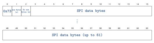
numBytes(n) specifies how many payload SPI bytes are contained in this packet (<=61)
