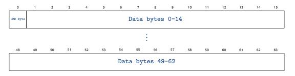
The CMD byte is a numeric literal which specifies the command. A command message may have up to 63 additional data bytes associated with it depending on its purpose. A description of each command is given below along with the format of a device responses if applicable. The device response will prefix its response in byte 0 with the CMD byte xor-ed with 0x80, i.e. it will send the command byte back with the MSB set to '1'.
