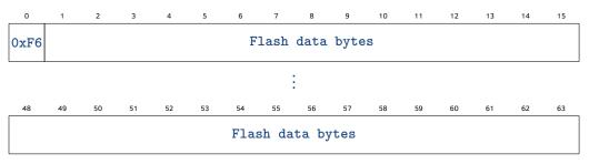
byte 1 is data as read from Address [31:0] byte 2 is data as read from Address [31:0]+1 and so on
