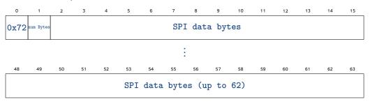
numBytes(n) specifies how many payload SPI bytes are contained in this packet (<=62) each byte in the desired SPI transfer follows up to the specified numBytes.
