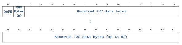
numBytes(m) specifies how many response payload I2C bytes are contained in this packet (<=62)
