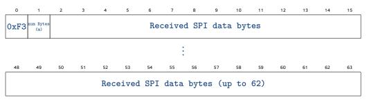
numBytes(m) specifies how many response payload SPI bytes are contained in this packet (<=62)
